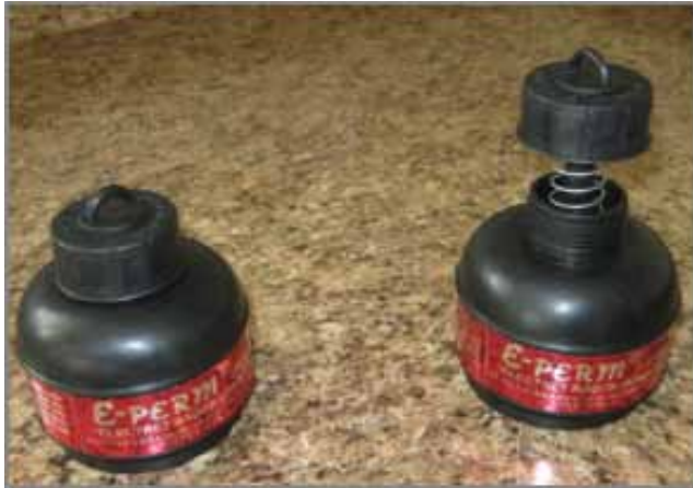
Image 1 – E-perm radon test devices
