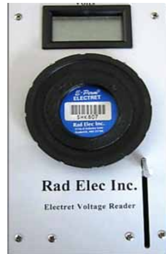
Image 2 – E-perm electret voltage reader
